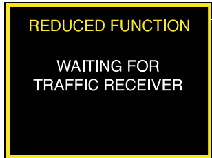
Figure 1.10.: After ATD has been switched on, this screen is shown until data from a connected traffic receiver is available
